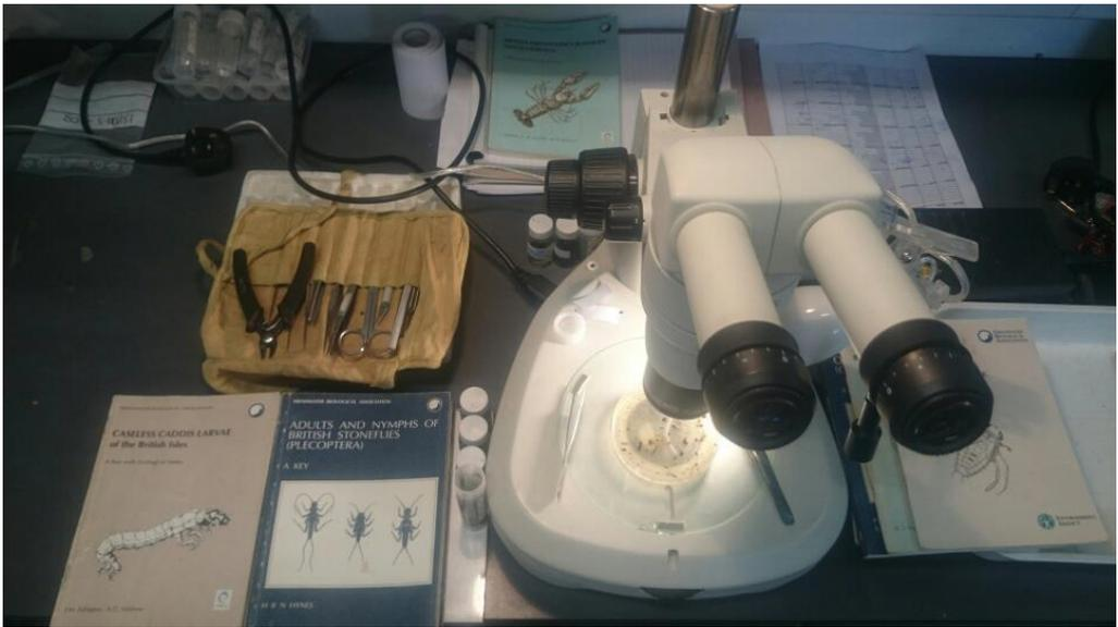
**Plate 1 – Nikon SMZ1000 microscope with LED lighting used in the identification of samples**
